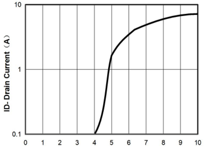
Figure8: Vgs Gate-Source Voltage (V)
